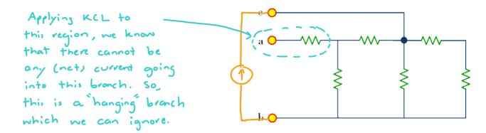
From the point of view of terminals b-c, the circuit is
